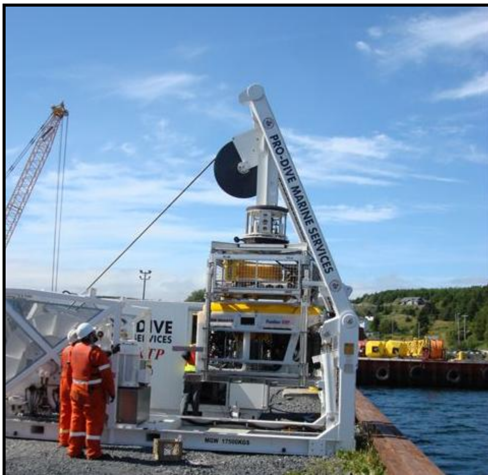
Panther XTP A-Frame LARS and TMS with Snubber Rotator
