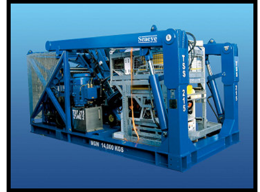
LARS in stowed position with TMS and Cougar ROV ready for transport.
